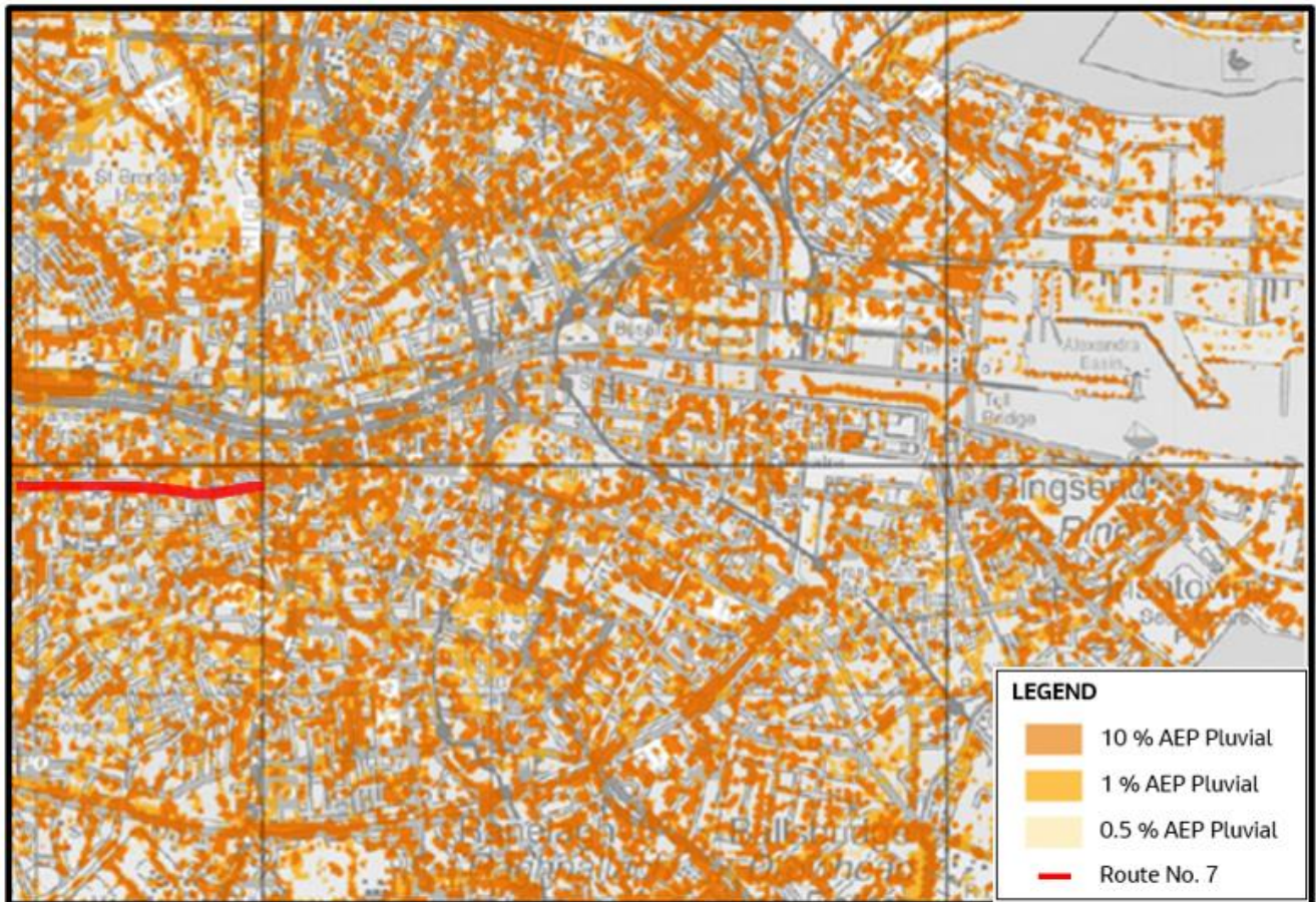
Figure 4.17 Extract of pluvial flood mapping on the Route No.7 bus corridor Kilmainham to City Centre
